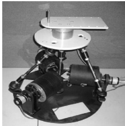
Figure 9. 3-RSS/S Ankle rehabilitation parallel Robot. Copyright IEEE. Reprinted with permission.
