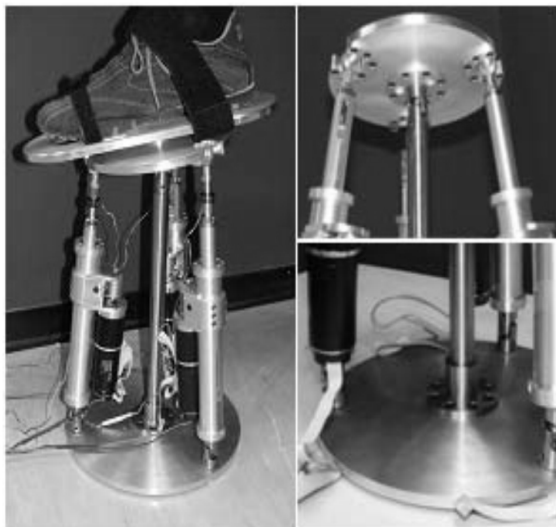
Figure 10. Prototype of 2 DOF over-actuated ankle rehabilitation robot [41]. Copyright IEEE. Reprinted with permission.
