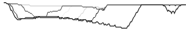
Figure 10. Pushback or economic limit as generated by the EP tool in 2D
