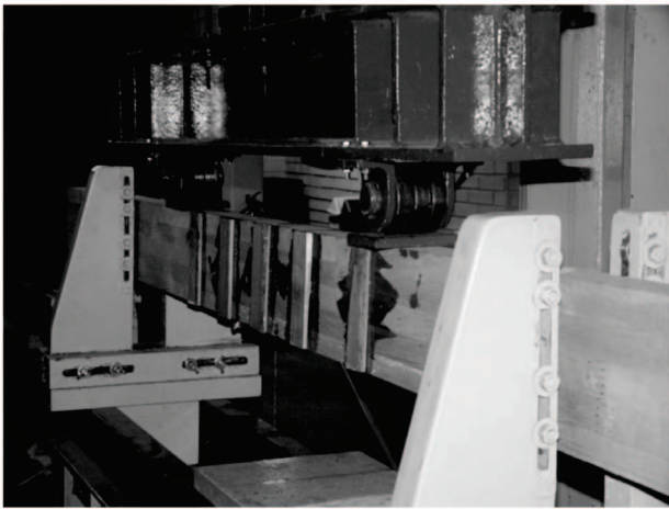
Figure 5. Bamboo-reinforced glulam beam
