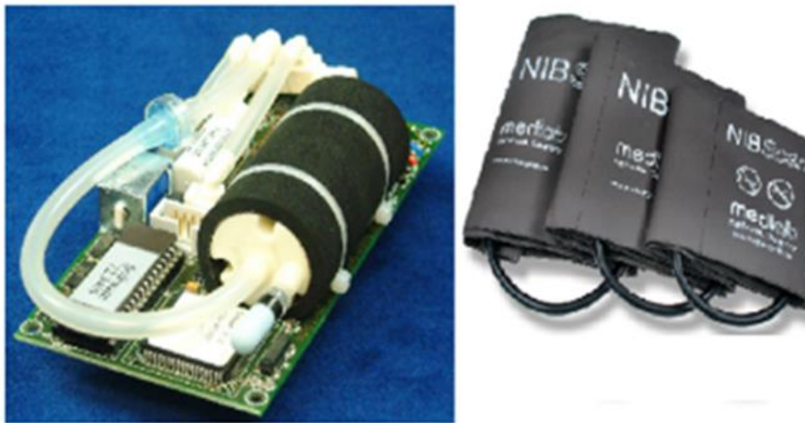
Figure 7. Electronic components for measuring PA [15].
