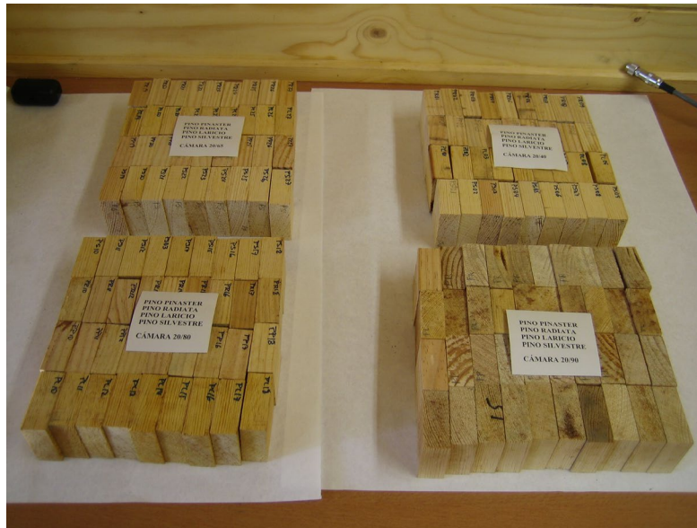
Figure 1. The four groups of specimens used in the study: above from the left 20/65 and 20/40 P. pinaster , P. radiata , P. laricio and P. sylvestris specimens, below from the left 20/80 and 20/90 specimens of the same species
