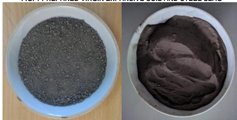
FIG. 1 PREPARED VIRGIN EXPANSIVE SOIL AND STEEL SLAG
