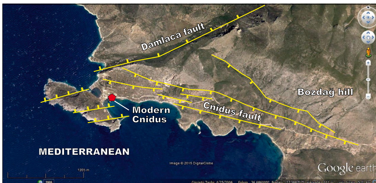
FIGURE 3. Google Earth satellite image, showing NE- and NW-trending normal faults located at the Modern Cnidus city (modified from Dirik et al. , 2003; Dirik, 2007).
