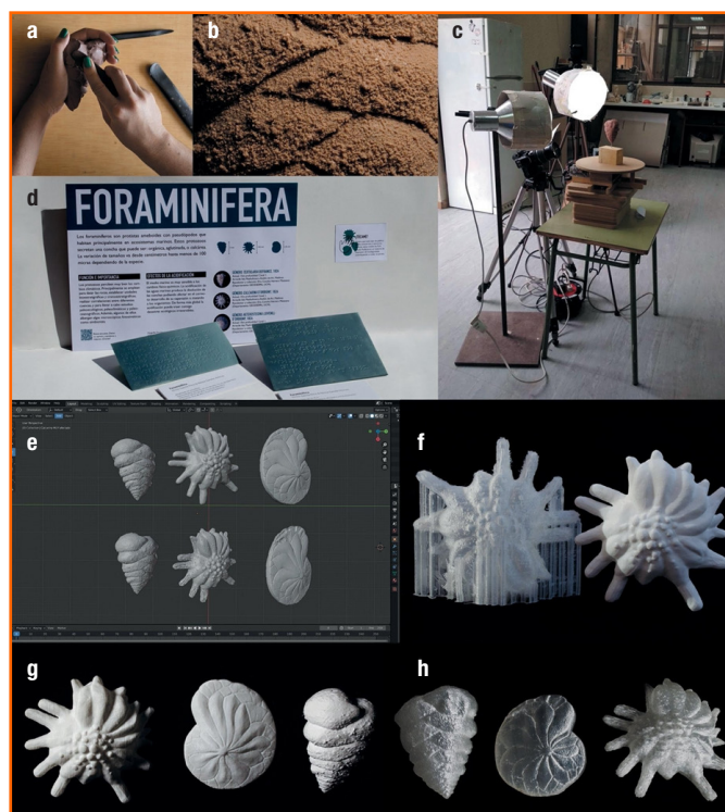
Figure 3. Creative process: (a) Clay modeling. (b) Textularia 's wall surface detail. (c) Layout for Textularia photogrammetry in the "set". (d) Explanatory and inclusive signage. (e) View of models (upper three healthy and lower three with corrosion and dissolution) in interface of Blender. (f) 3D print with supports and 3D clean print of Calcarina . (g) 3D healthy prints of Calcarina , Heterostegina and Textularia . (h) 3D prints with acidification effects of Textularia , Heterostegina and Calcarina .
