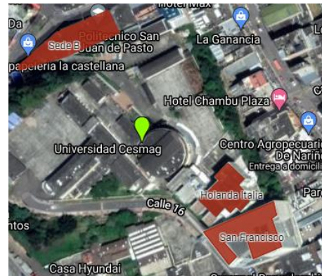
Fig. 6. Available areas for PV roofs within the University Campus.
