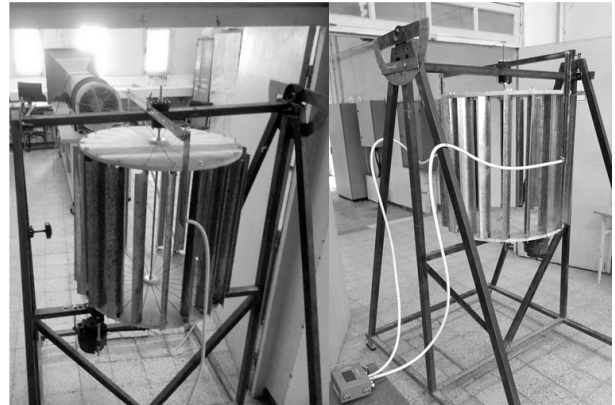
Figure 2. Experimental setup of the vertical axis wind turbine Source: The authors
