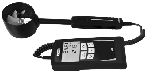
Figure 6. LVA thermo-anemometer Source: The authors
