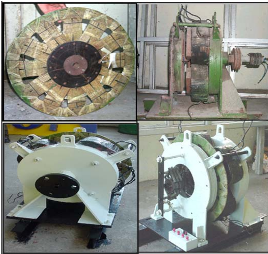
Fig. 3 Synchronous generator of low reversibility 12,5kVA / 10kW / 4 poles.
