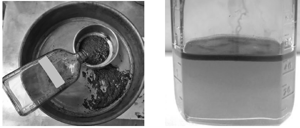
Figure 1. Corrosion inhibitor effect on sludging trend & acid dispersion. Source: The authors.
