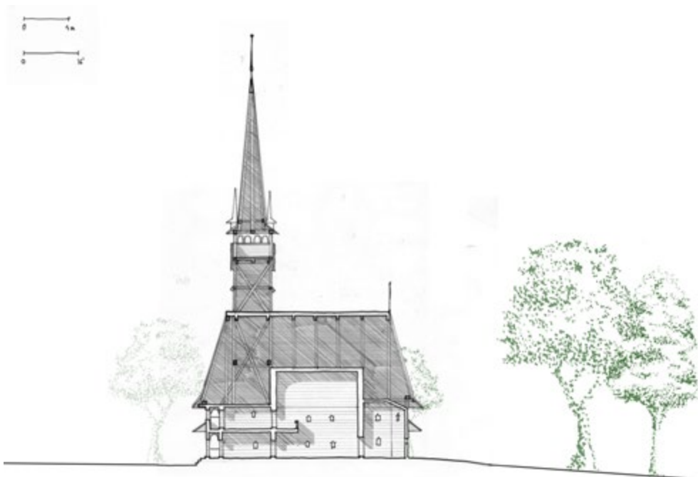
Section of the Church of Archangels Michael and Gabriel in Șurdești, Romania
