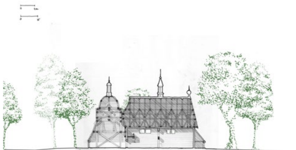
Timber frame and Blockbau , Church of St. Philip and St. James in Sękowa, Poland
