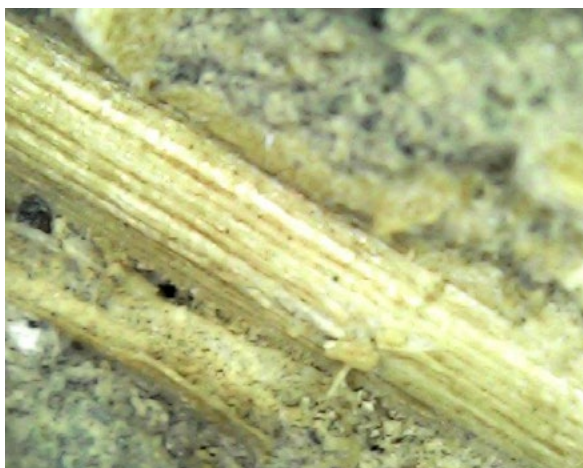
Figure 11: 1000x microscopic image of the earth and fiber layer of the CAR02A sample (Manuel Concha)
