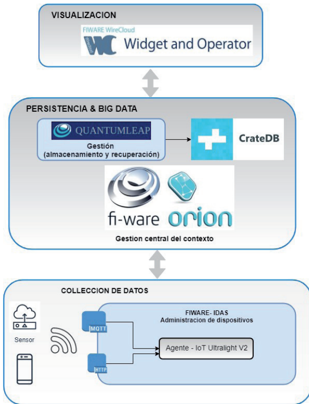
Figure 5: IoT solution architecture based on FIWARE.
