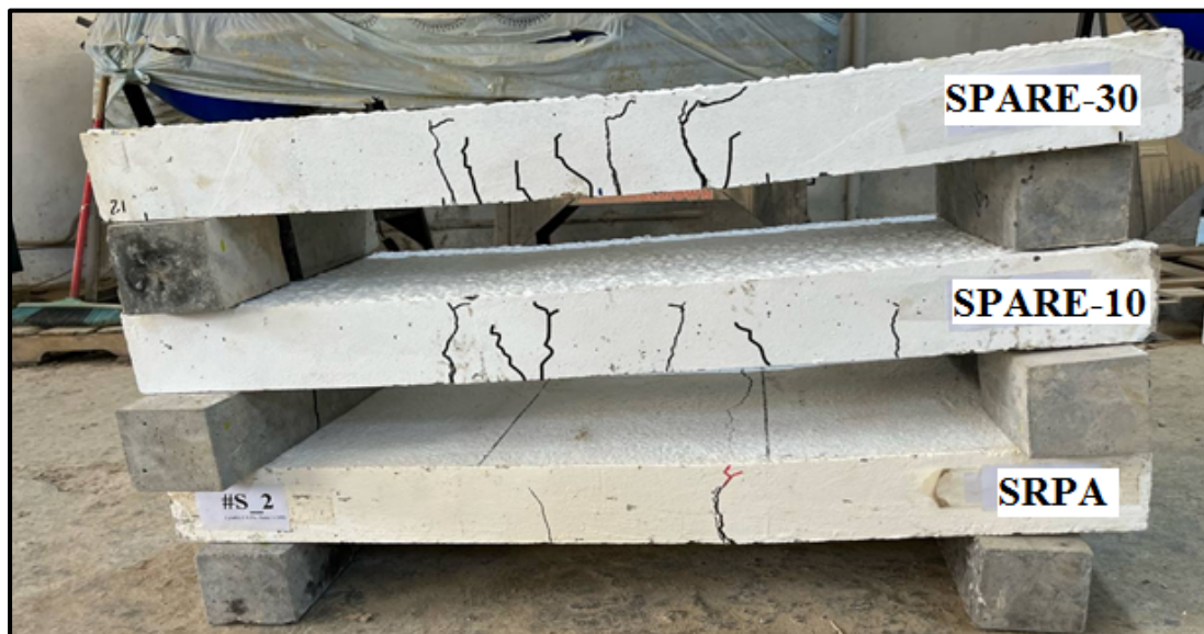
Figure 11. Crack pattern for the HCS specimens of Group Two.
