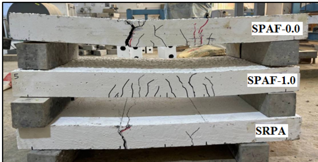
Figure 10. Crack pattern for the HCS specimens of Group one.
