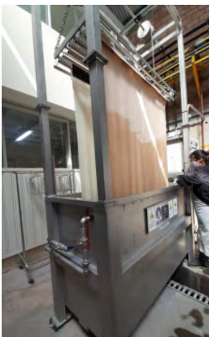
**Figura N° 2.** Máquina Deep Dyeing 50 instalada
