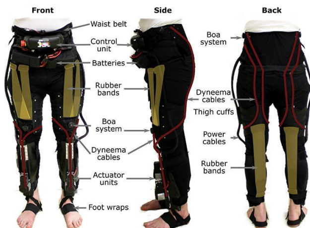
Figure 4. MYOSUIT exoskeleton [15].
