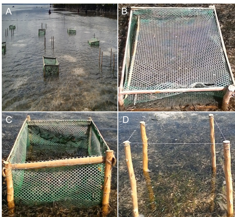
Figure 2. Different caging treatments in the study site (A), full cage (B), partial cage (C), and open cage (D).
