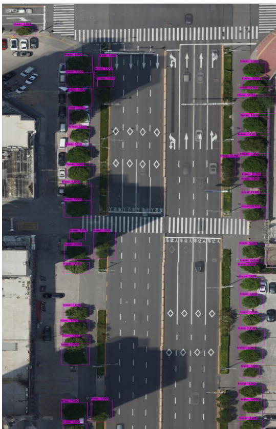
Fig. 6. Detection results of straight road scene.
