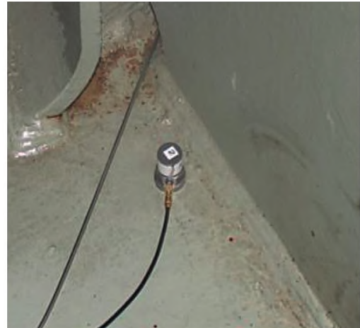
Figs. 8 and 9. Accelerometer placed in the ship structure.
