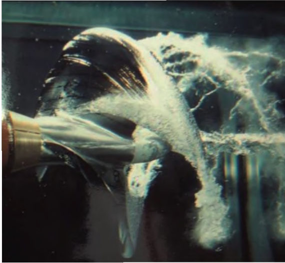
Fig. 3. Cavitation in naval propeller.
