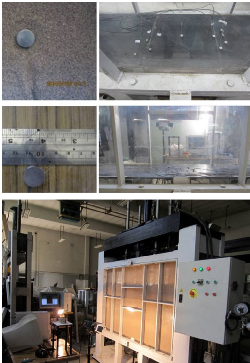
Figure 2. Built physical model and used strain gauges
