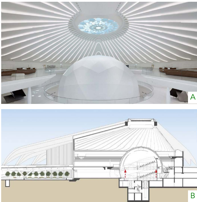
Figure 13. (A) UAE pavilion spherical core and (B) its section. Source: Ravenscroft, 2021.
