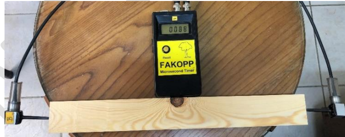
Figure 4: Measuring time of flight with Fakopp micro second timer.
