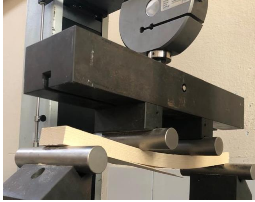
Figure 10: Brittle tension rupture of structural timber board.
