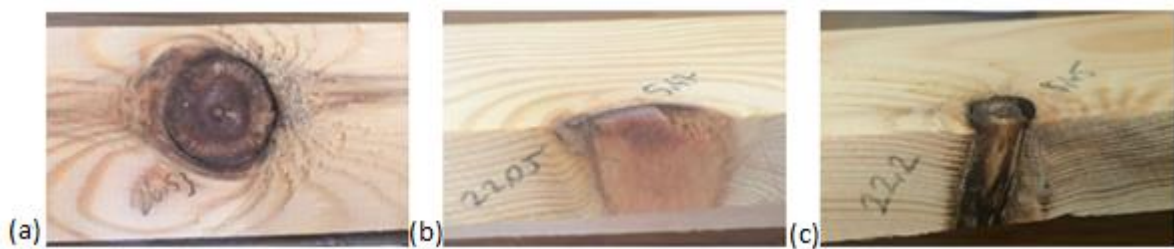
Figure 7: Knot locations (a) at the wide face (b) big knot and (c) small knot at the narrow face.
