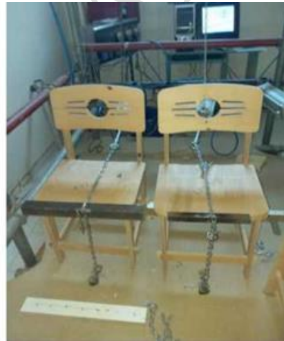
Figure 7: Front to back loading performance testing of chairs.
