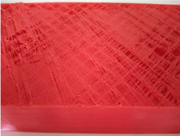
Fig. 21: Stop extruding the plastic without finishing the print. (Self made)
