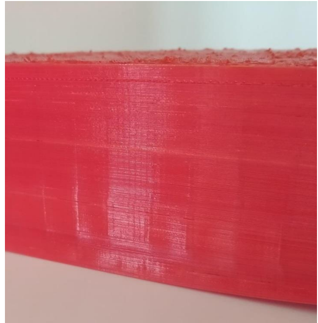
Fig. 26: The inner filling is perceived on the surface. (Self made)
