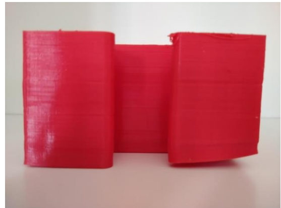
Fig. 17: Warping, front view. (Self made)
