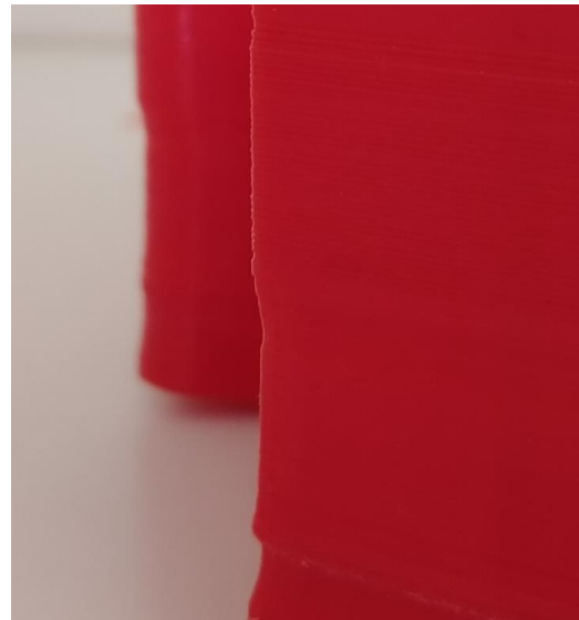
Fig. 20: Layer displacement. (Self made)
