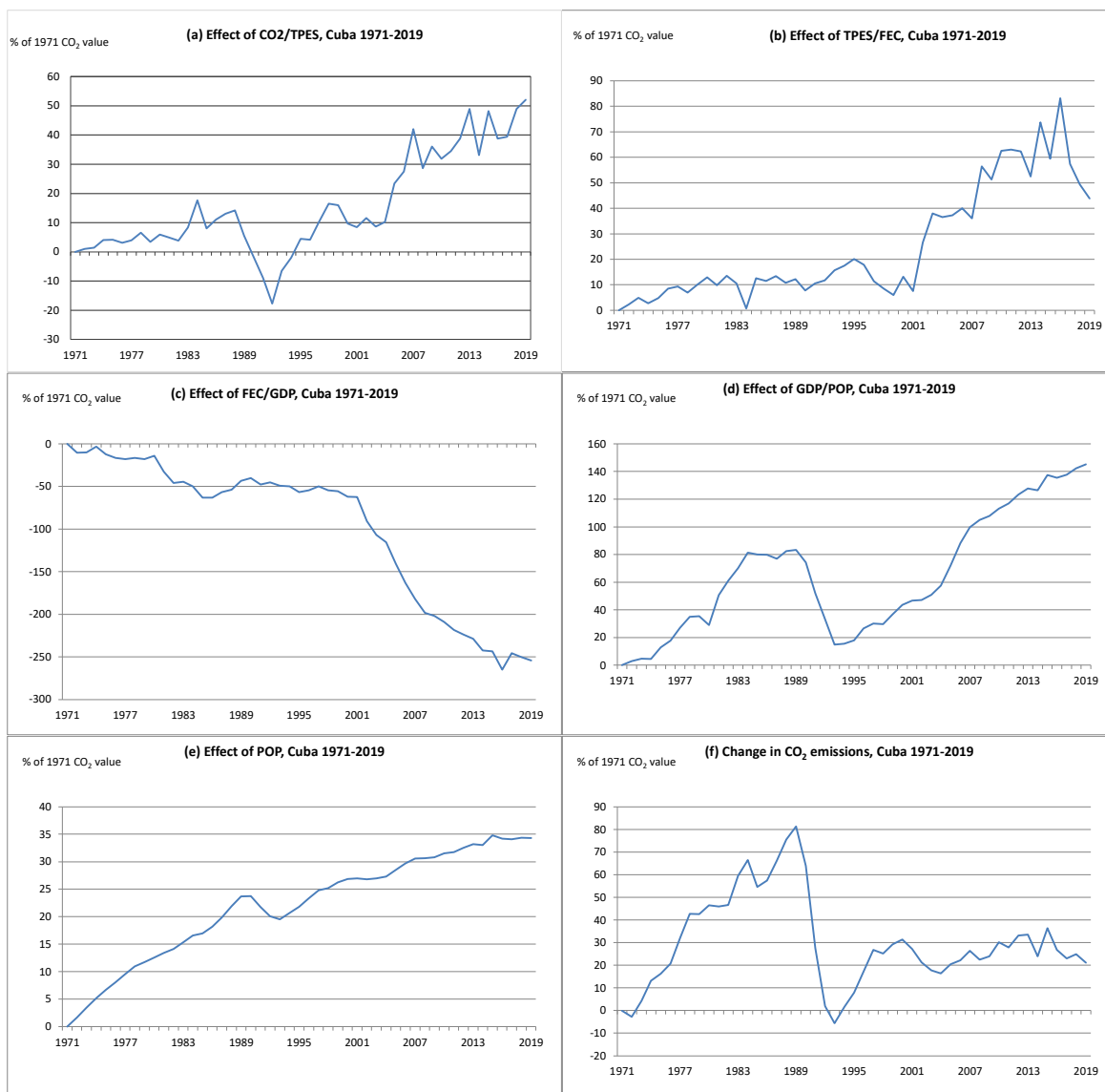
Fig. 4. Impact of the extended Kaya identity factors CO 2 /TPES (a), TPES/FEC (b), FEC/GDP (c), GDP/POP (d), and POP (e) on change in CO 2 emissions in Cuba 1971–2019 (f), as a percentage from the base year 1971 CO 2 value. Data sources: IEA [28], UN [29]
