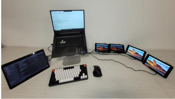
Figure 4. Setup for emulating the proposed power aggregator: left) Raspberry Pi + screen, right) computer with Matlab Simulink for the emulation of the active-distribution network. Source: self-made.
