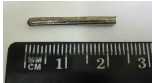
Figure 1. BMG rod obtained by copper mold casting.
