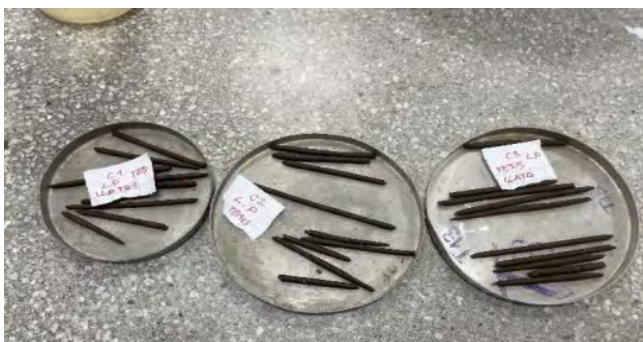
Figure 2. 3.2 mm thick bars to determine the PL of C-3 clay soil samples. Source: self-made
