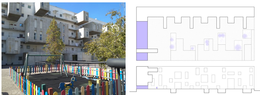
Figure 9. 102-unit social housing project ( dosmasunoarquitectos ). General courtyard and ground floor schemes (floor plan and section) of common spaces
