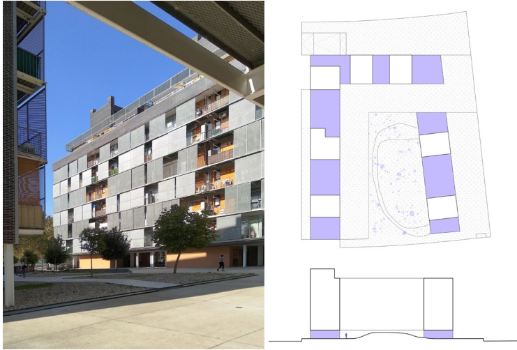
Figure 4. 78-unit social housing project (Jacobo García-Germán). General courtyard and ground floor schemes (floor plan and section) of common spaces
