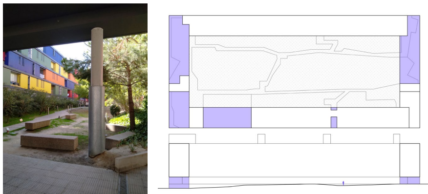
Figure 8. 82-unit social housing project ( temperaturas extremas ). General courtyard and ground floor schemes (floor plan and section) of common spaces
