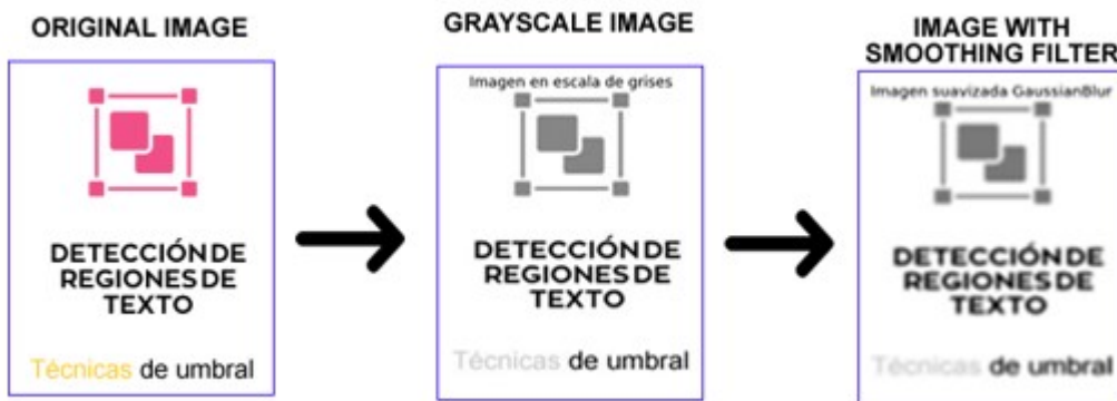
Figure 4. The result of applying a combination of preprocessing filters to the original image Source: own elaboration.
