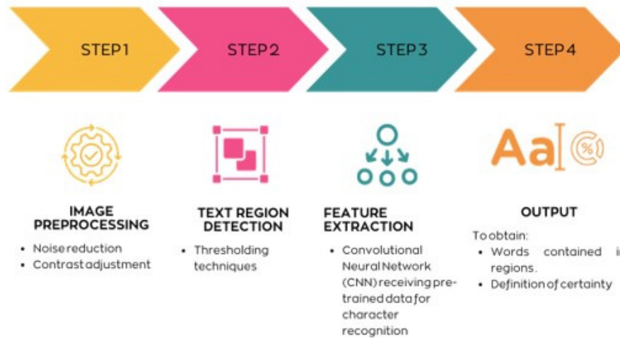
Figure 3. Steps to be carried out for reading and extracting text from images.
