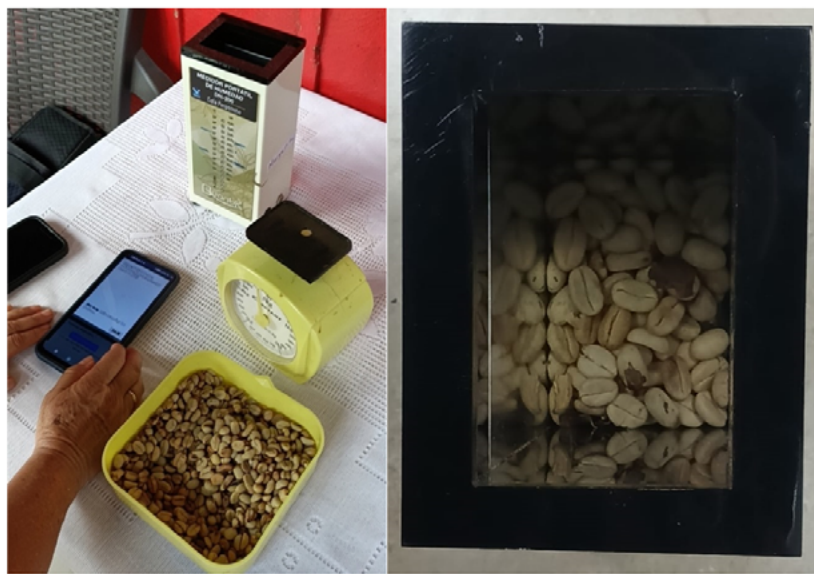
Fig. 3. Sample measurement setup: Users must select a 200-gram sample and place it inside the DH-200. The device transmits the data captured to a cell phone via Bluetooth.
