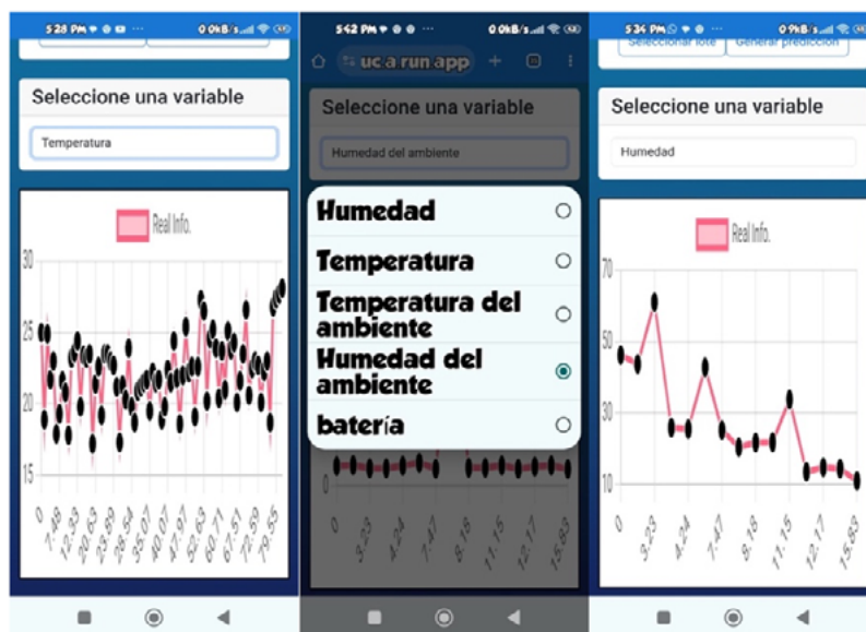
Fig. 6. Mobile app interface of the IoT for analyzing the coffee drying process. From left to right: selection of the plot of temperature, center, interface to select a variable, and selection of the plot Humedad (moisture of the coffee bean).
