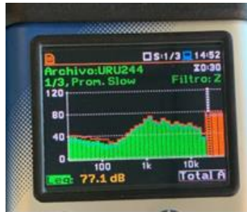
Figure 3. Svan 977 Sound Level Meter setting
