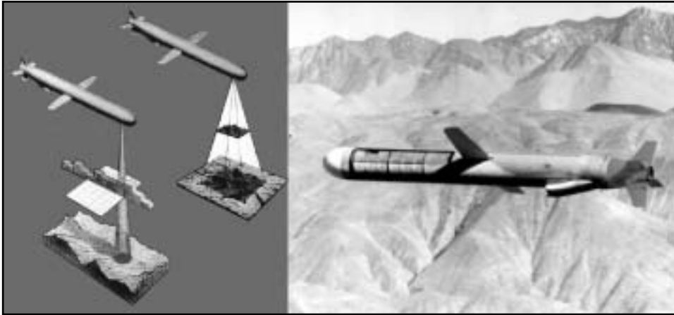
Figura 33. Misil Tomahawk. 1. DSMAC (Digital Scene Matching Area Correlation). 2. TERCOM (Terrain Contour Matching Radar).
