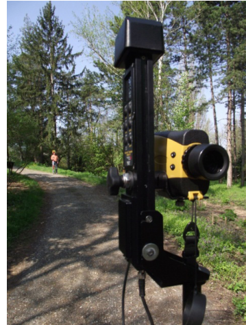
Figure 2 The MapStar Compass Module II and TruPulse 360B
