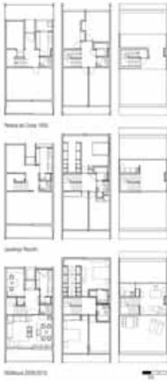
Figure 8: The duplex – fourth case study – floor plan. The original distribution, top, the first intervention, middle and the current stage, below.
