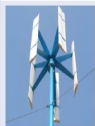
Vertical Lift Axis (Darrieus)
