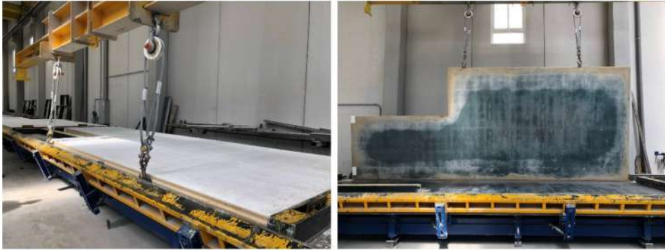
Figure 12. Lifters to remove the plates from the mold 72 hours after pouring.
