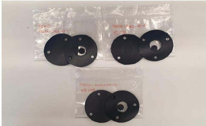
**Figure 39.** Test samples of different percentage of CNT.
