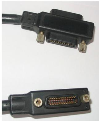
**Figure 30.** GPIB IEEE-488 Connector.
