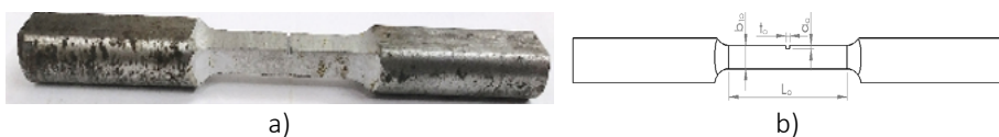
Figure 1. Rectangular cross section specimen to realize the cyclic torsional test. a) Pre-cracked specimen. b) Dimensions in the section where the pre-crack was machined.
