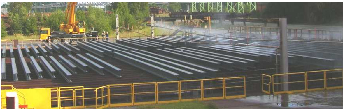
Figure 14. PTG’s cooling bed. Picture courtesy of BFI.
