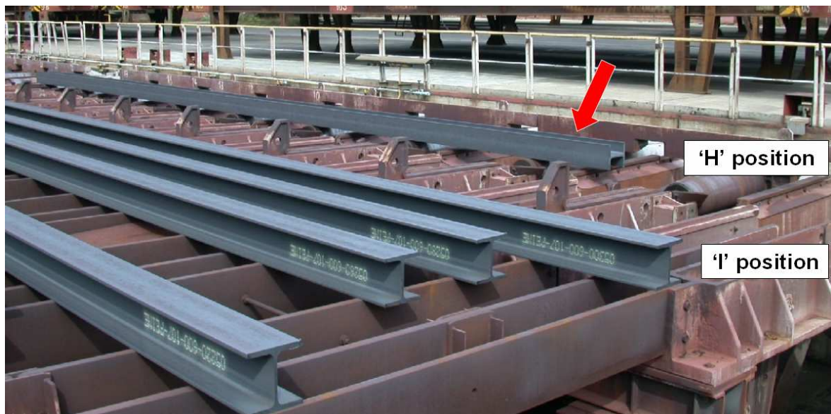
Figure 27. Input part of the cooling bed studied for the H profiles. Picture courtesy of PTG.
