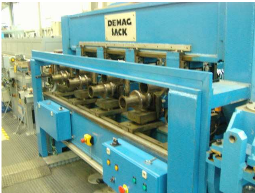
Figure 88. BFI's Hot Straightening Machine (HSM). Picture courtesy of BFI.
