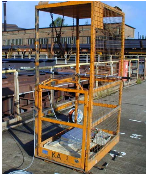
Figure 20. Crane's cage with measurement equipment.
