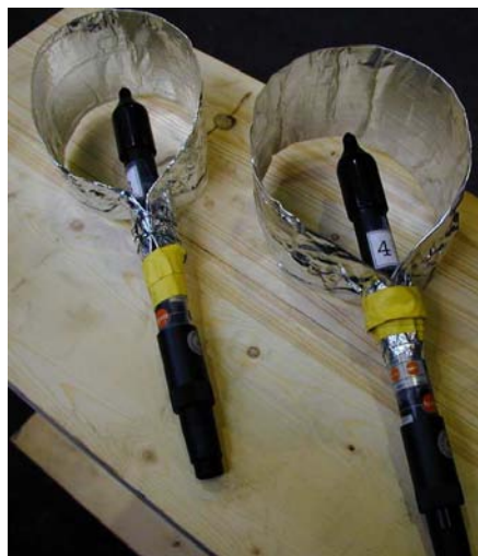
Figure 17. TESTO® 3-function probes with a cover to measure unidirectional wind speed.
