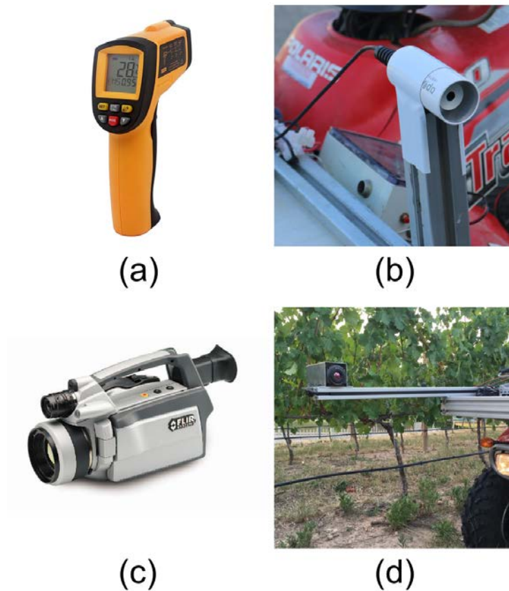
Figure 1.11: Different examples of devices for IR thermal sensing. (a) A thermal IR gun that requires manual operation. (b) A IR radiometer, capable of carry out automatic, continuous temperature monitoring. (c) A handheld thermal camera. (d) A compact thermal camera for automated imaging. Source: FLIR Systems and Televitits research group, University of La Rioja .
