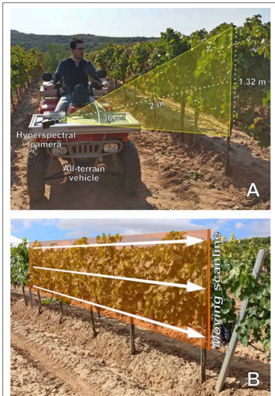
FIGURE 1 | (A) On-the-go hyperspectral imaging on an all-terrain vehicle in a vertically shoot positioned vineyard located in Logroño, La Rioja (Spain). Spectral acquisition was performed on the sun-exposed canopy side at 5 km/h. (The authors declare that written and informed consent has been obtained from the depicted individual in this image, for the publication of this identifiable image). (B) Construction of a two-dimensional hyperspectral image by push broom. The camera's scanline, that was acquiring spectral information from a vertical line over the vineyard canopy, was moved by the motion of the all-terrain-vehicle. Thus, the composition of the image was performed by this scanline dragging at constant speed.
