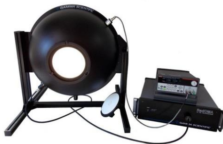
Figure 2.3. Spectroradiometer composed by a big integrating sphere (left) and a detector (right), (commercial RadOMA equipment).
