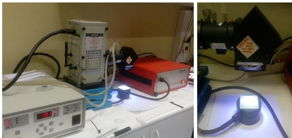
Figure 9.3. Solar simulator and experimental setup for SPF measurements.
