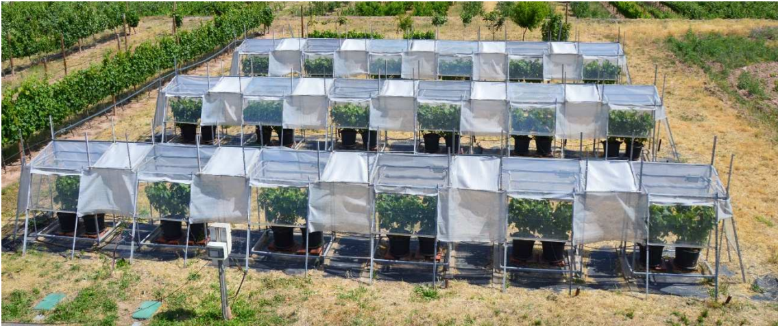
Figure 7.2. Experimental set-up at Universidad de La Rioja, which consisted of 18 blocks arranged in three parallel rows. Transparent specific cut-off filters covering each block and white shading mesh in the gaps between blocks can be seen. Two grapevine plants were placed in pots in each block.
