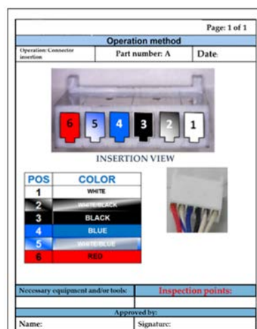
Figure 6. Provisional aid for cable insertion.
