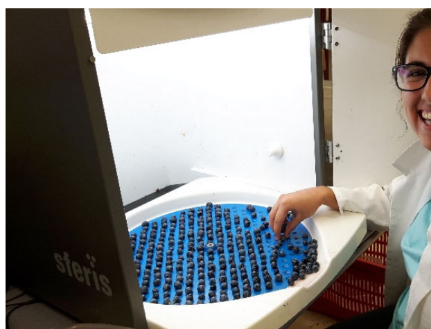
Figure II-2. 1. Dyostem ® (Vivelys, France), tool for evaluating the enological potential of plots and determining the harvest date.
