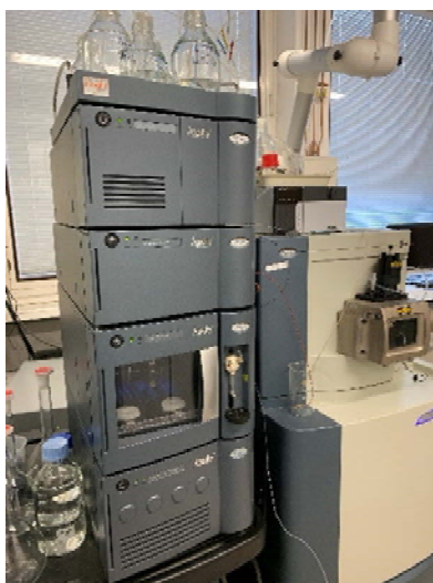
Figure III-3. 1. Chromatography system. Waters Acquity UPLC coupled Synapt HDMS QTOF MS (Waters, Manchester, U.K.)
