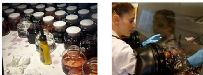
Figure IV-3. 5. Experimental process: Left, caps sealing with glue to ensure complete airtightness; Right, fractions keeping in the anoxic glove chamber from Jacomex (Dagneux, France).
