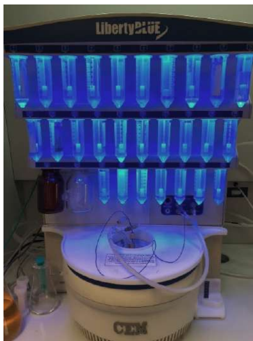
Figure 4.3. Liberty Blue synthesizer used for this work.
