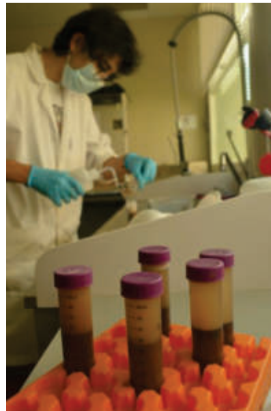
Figure 26. Tubes with sieved soil samples ready for the sucrose centrifugation procedure. Photo by Rubén Blanco Pérez from Instituto de Ciencias de la Vid y del Vino, Spain.
