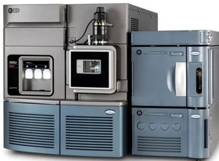
Figure 3-3. UPLC-MS instrument coupled to Q/TOF mass analyser.
